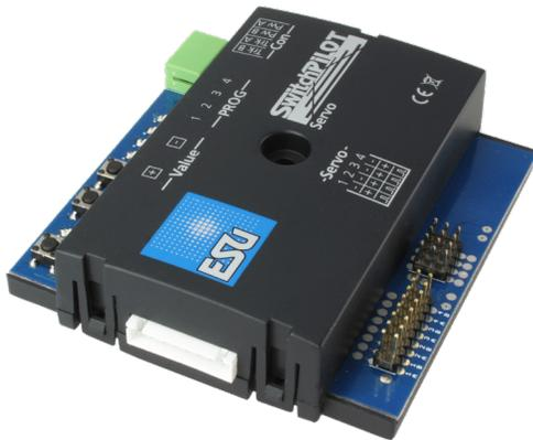
For each servo, not only lever speed can be adjusted individually but also its end positions. Thus it is possible to operate especially prototypically slow and powerful turnout motors, independent of track- and gauge systems. You could also employ the SwitchPilot Servo for driving Semaphore Signal arms or railway crossing gates. Also the automatic opening of engine house doors does not need to remain a dream.
