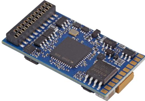
The LokSound 5 is the most important member of the LokSound family. Due to the combination of digital decoder and sound module on a printed circuit board, the decoder is only 30mm x15.5mm and can be installed in almost any locomotives of in H0, S, or 0 gauges if the max amperage draw is under 1.5 amp.
