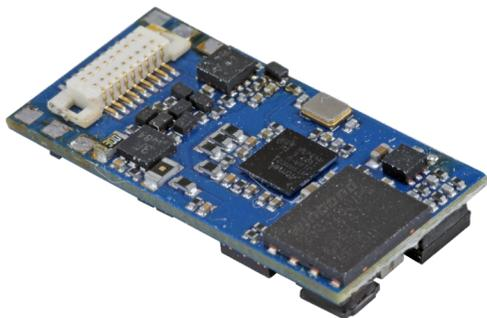
The LokSound 5 micro is a “little wonder”: With only 21mmx10mm footprint, it is by far the smallest LokSound decoder we’ve ever built. This is perfect for N scale, but can also be used in small H0 locos. LokSound 5 micro decoders always have a Next18 interface and are offered with adapter plugs for all common interfaces.
