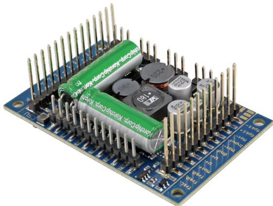
The LokSound 5 XL decoder is an extremely powerful decoder! It must be as it is intended for use in your garden railway or gauge 1/G gauge locomotives. Its integrated, power-adapted PowerPack ensures safe operation even on dirty tracks.
