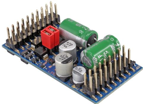
The LokSound 5 L finds its place in O Scale between the LokSound 5 and the LokSound 5 XL. With dimensions of just 51mm x 25.5mm, it is not only recommended for size 0 scale locomotives, but also for all other models where a LokSound 5 XL does not fit or is required.
