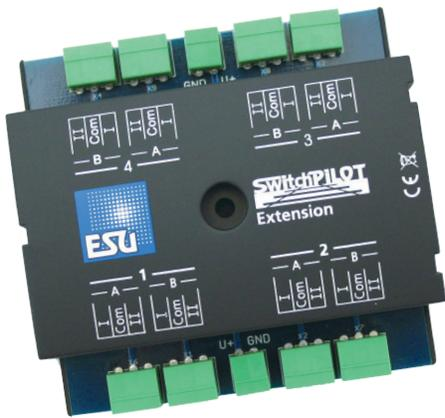
If required, SwitchPilots and SwitchPilot Servos can be augmented with the SwitchPilot Extension Module: Plugged in at the side of the SwitchPilot, it offers four relay-driven outputs, used for switching potential-free loads, or for polarizing the frog; the ideal supplement for tricky circuitry.
