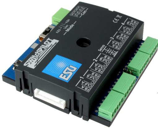
The SwitchPilot 2.0 is an updated version of our well known accessory decoder. It is a robust multi protocol switch and accessory decoder for controlling up to 4 solenoid accessories (e.g. Switches) or 8 loads such uncoupling ramps or incandescent lamps (e.g. street lighting, lighting of buildings or signals). Due to its intelligent software it can be operated with any DCC system.
