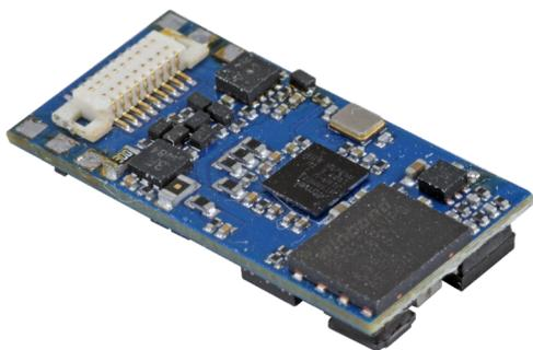
The LokSound 5 micro is a “little wonder”: With only 21mmx10mm footprint, it is by far the smallest LokSound decoder we’ve ever built. This is perfect for N scale, but can also be used in small H0 locos. LokSound 5 micro decoders always have a Next18 interface and are offered with adapter plugs for all common interfaces.
