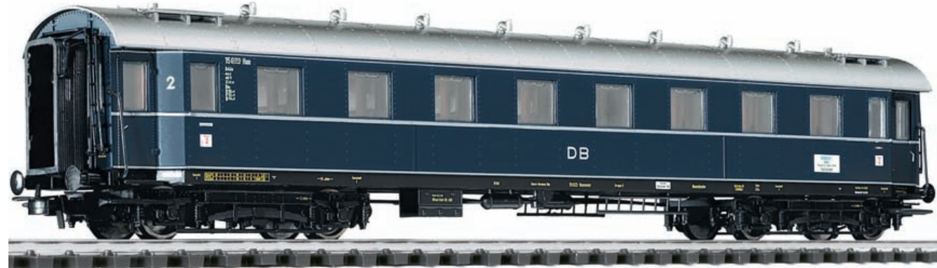
F-Zugwagen 2. Klasse, DB, Epoche III Bauart B4üe-30/52, Federpuffer, LüP 250 mm.
