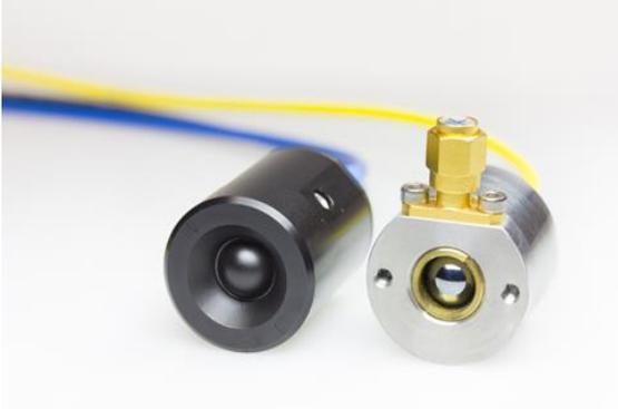
Fig. 5: Photomixers with fiber pigtailed. The active structure sits at the center of the cylindrical package; the generated terahertz radiation is emitted through the silicon lens.
