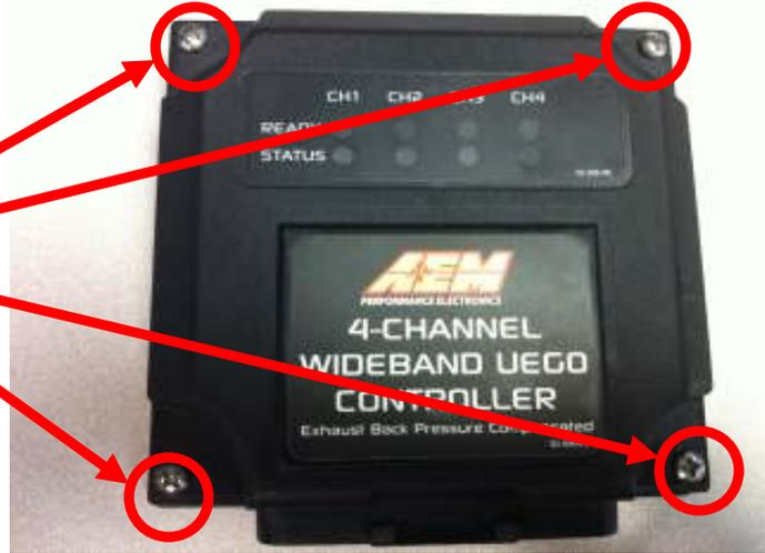
**FIGURE 3. Mounting holes**
