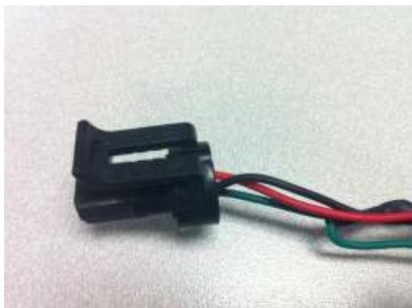
Figure 6. EBP sensor connector
