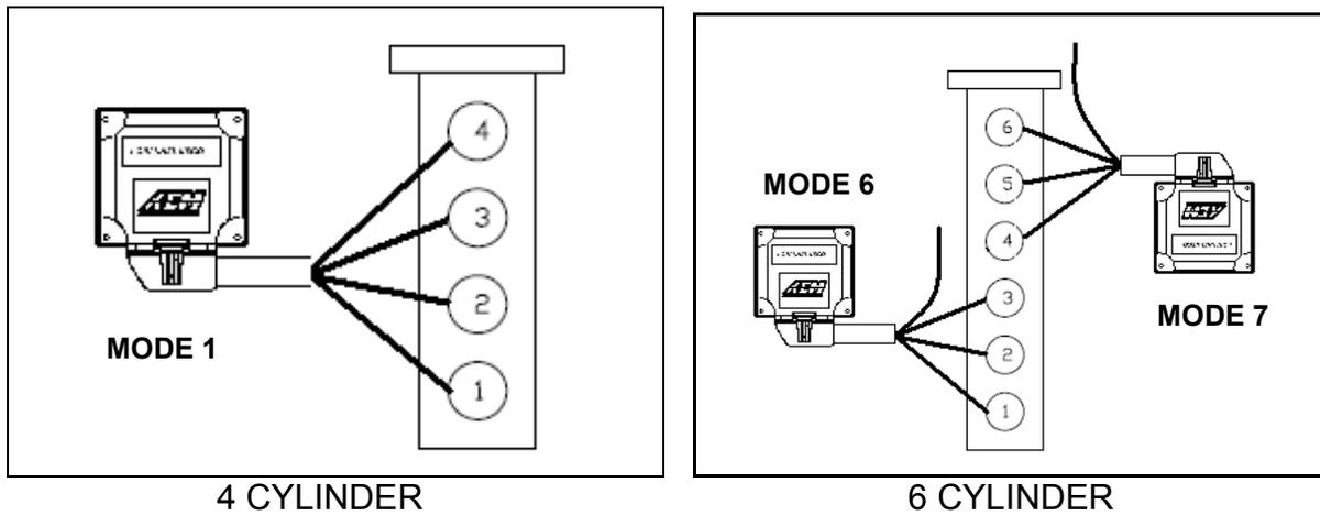
**FIGURE 8. 4 CH UEGO controller configuration mode**
