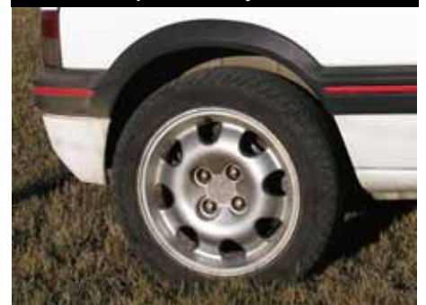
Above: Series 1 & 2 GTis had 14 inch "Pepperpot" alloys fitted. Series 3 cars came with 15 inch 'Speedline' alloys as below.
