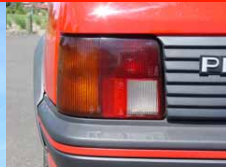
Above: The Series 1 tail lights incorporated a reversing lamp. The series 2 and 3 cars had a separate reversing lamp.
