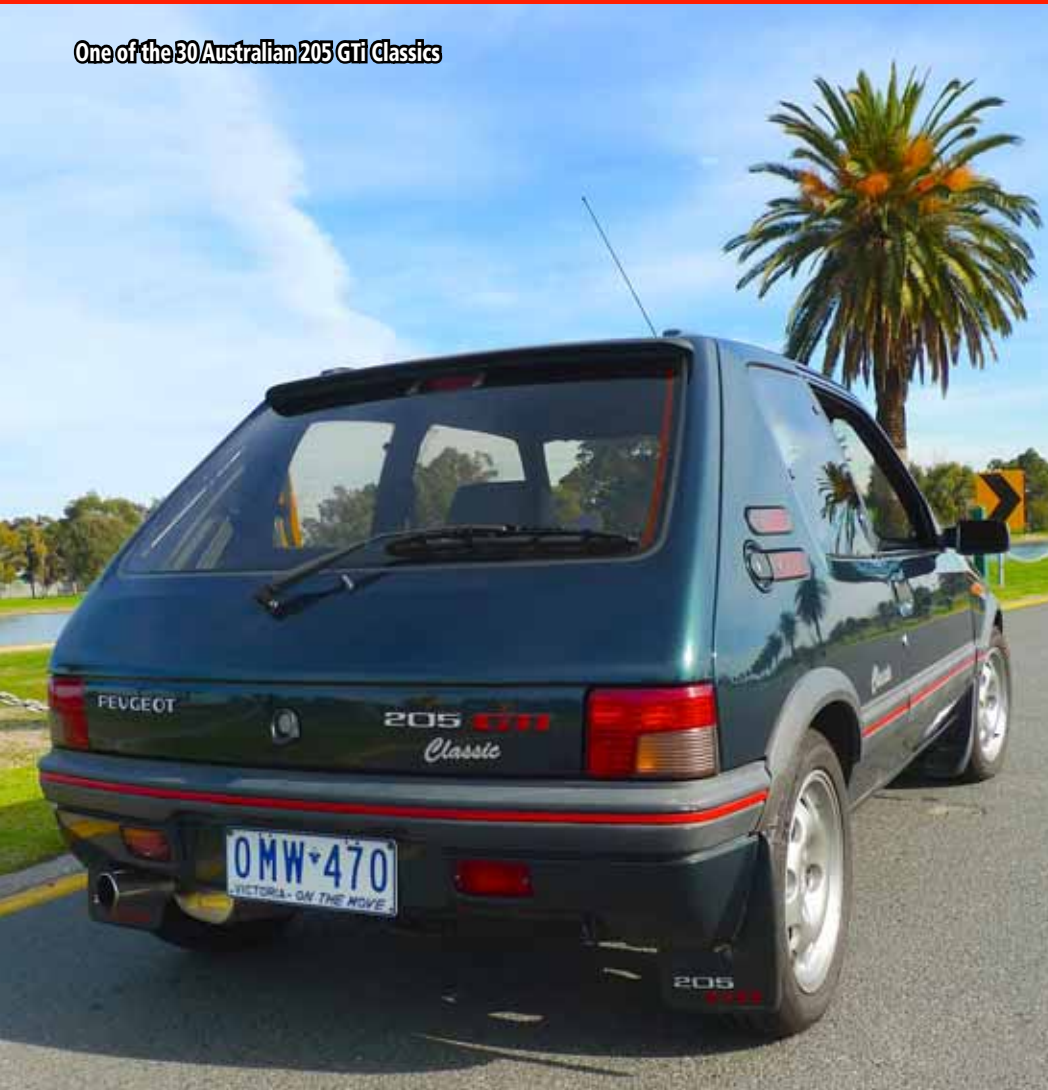
Above: The Series 1 tail lights incorporated a reversing lamp. The series 2 and 3 cars had a separate reversing lamp.
