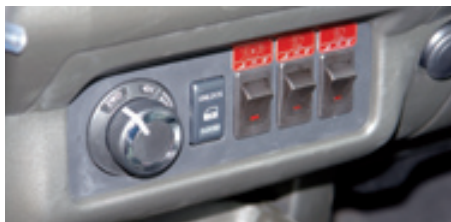
La commande de transmission. The transmission controls
