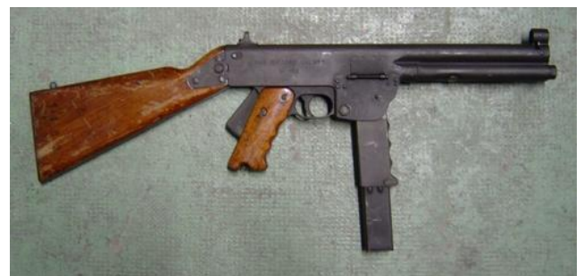
PM Mle 48 MAT prototype crosse bois repliable
