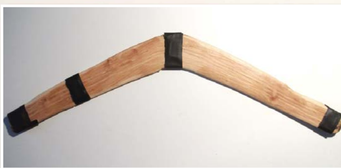
Fig 6. Replica weighted with lead fixed by adhesive tape (prepared for four strip test).
