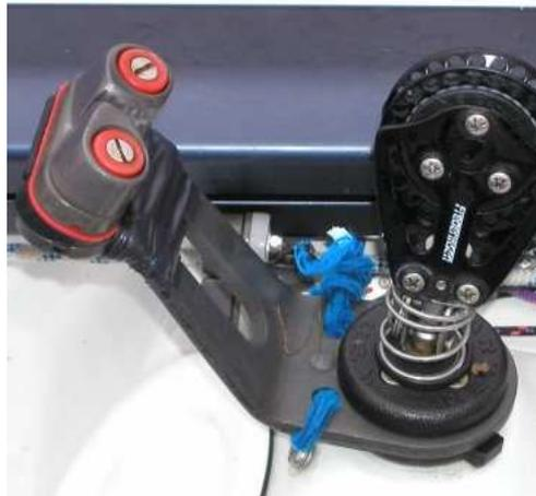
It's also worth considering replacing the standard strop block, with one of the new ones with a big hole in the middle. Then the mainsheet can be dead-ended with a stopped knot after going through the block, and you will be able to sheet more "block to block". This photo below shows a better block but uses a clunky knot, which eliminates all the benefits of the block.
