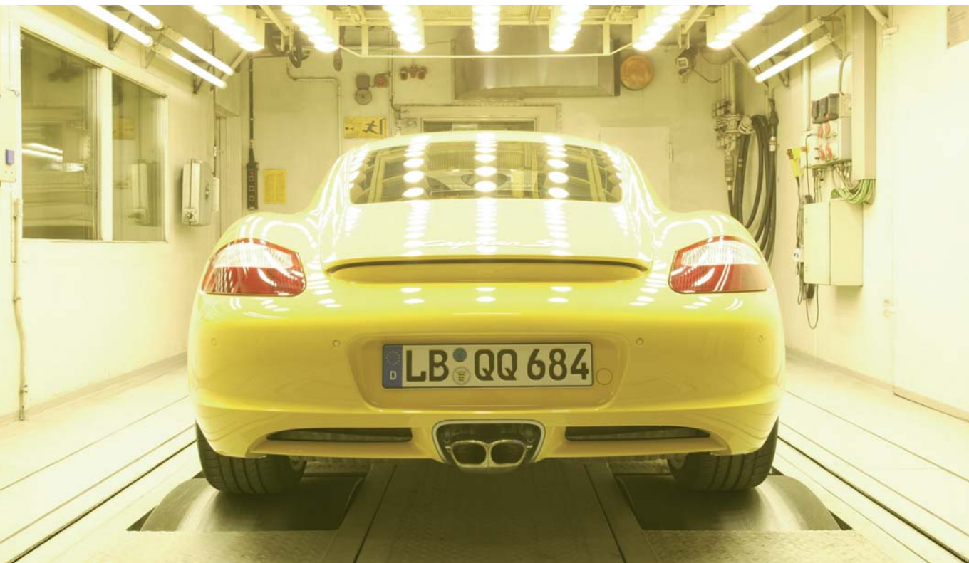
Cayman S in the climate wind tunnel at the R & D Center in Weissach. Real stretches of road can be simulated here under real climate conditions, such as the Townes Pass in the USA.
