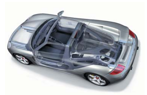
Apart from the monocoque and engine mount of the Carrera GT, numerous other components were made from carbon-fiber reinforced plastic (CFRP).
