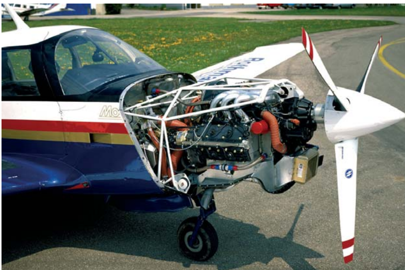
Porsche Type 3200 aero engine with 3.2-liter capacity.
