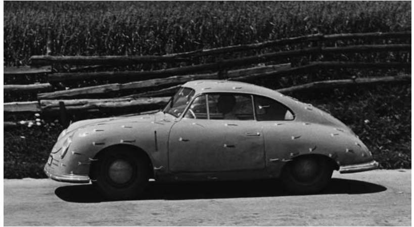
First aerodynamic tests were carried out on the Porsche 356 using pasted woolen threads.
