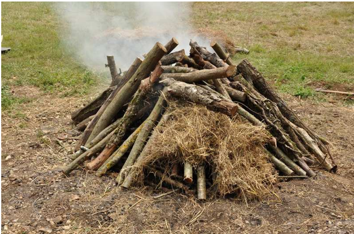
Figure 23 – montage de la meule - Cliché C. Albaret
