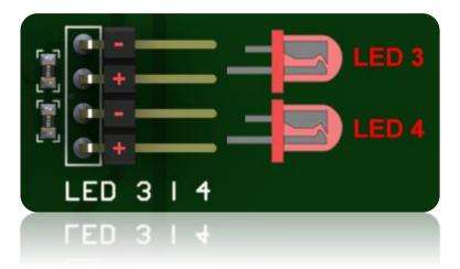
**Important**: You need some experience with soldering. Be careful and make sure you use proper isolation if going for soldering method.
