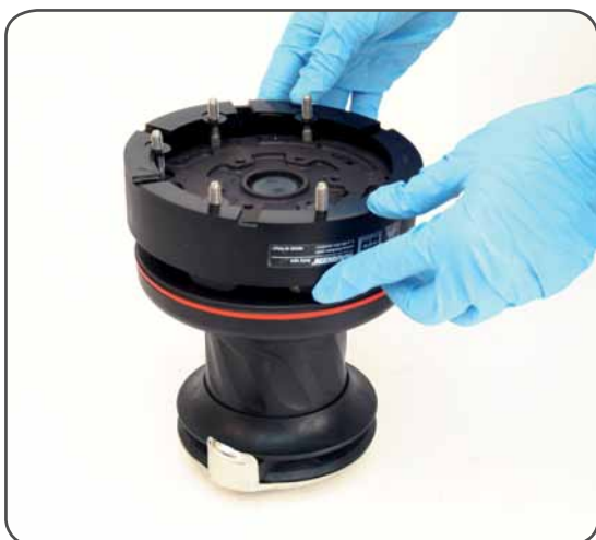
4. Reposition the skirt n°2 in its housing
