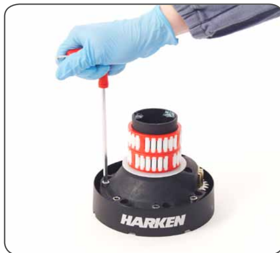
9. Unscrew the 6 hex screws n°16 (🔧 8Nm/71 in-lb)
