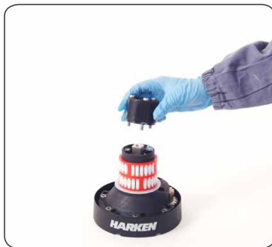
7. Remove the self-tailing arm support n°21
