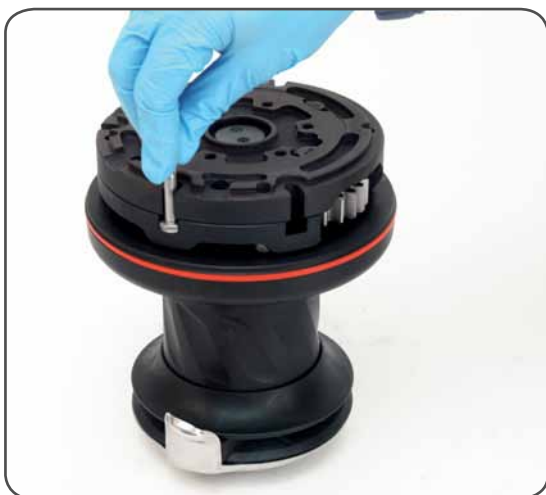
3. Position the 5 M6 hexagonal headed bolts in their holes
