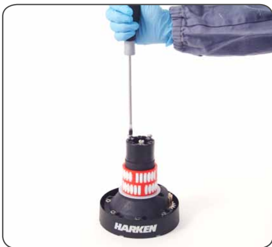
6. Completely unscrew the three screws n° 27
