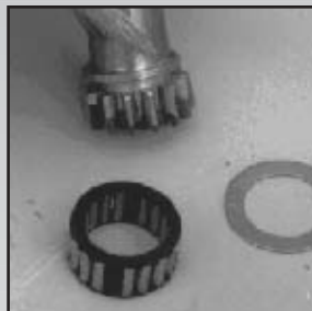
Clean all parts, except 37383 and 37339, with solvent.
