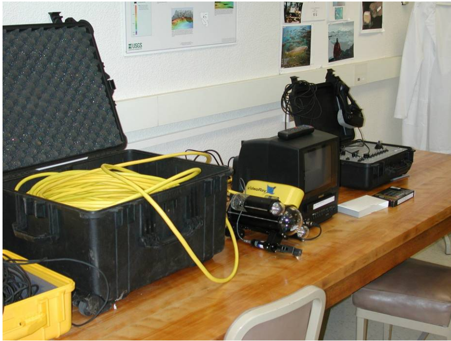
Figure 2. Remotely Operated Vehicle (ROV) with 152 m (500') tether
